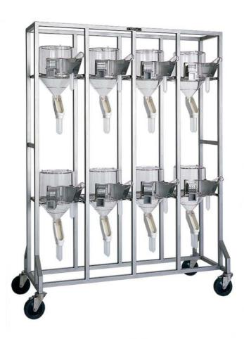
A space-efficient rack is available—as a separate item or as part of the complete system—that accommodates eight metabolic cages. Each cage is positioned on a removable shelf. Fabricated of heli-arc welded stainless steel with four 5" diameter neoprene casters (two with brakes). Size: 51.6" wide  $\times$  20.0" deep  $\times$  71.1" high (including casters and outriggers).
