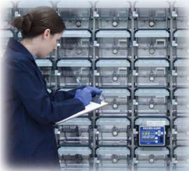
Certify Airflow with the Enviro-Gard™ Cage Monitor Control Unit and RAIR Enviro-Gard™ Airflow Monitor / Alarm Unit.
